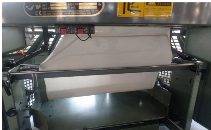
1-rasm. BAI YUAN to'quv mashinasida yopqichli namuna ishlab chiqarish jarayoni
